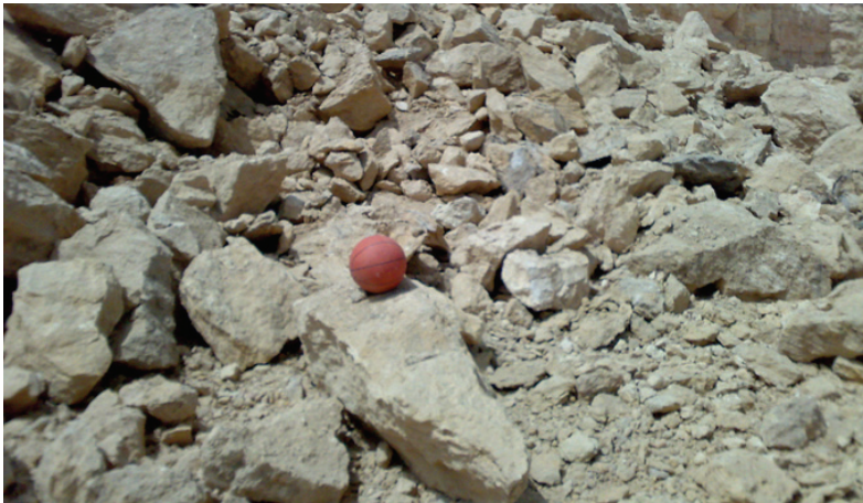
Fig. 2. Typical image taken in the field for calculation of size distribution.
